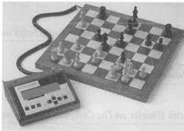
The R30 is the first CC to have an operating unit entirely separate from the board.
